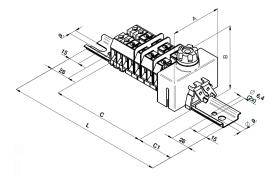
Fuse holders in pole terminal board systems do not include own fuse element (fuse D02) due to the varying requirements of customers for their own types of fuses. The E14 and E27 cut-out bases do not include a pressure insert (distance ring).
