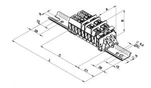
The terminal boards are clamping on the DIN Rail TH 35 from terminal blocks RSA 6, RSA 10 A, RSA 16 A or RSA 35 A, including the accessories, and they can be used in the TN-C and TN-S system. The basic version includes a cut-out base (fuse terminal block RSP 4). It is possible to order terminal boards with several cut-out bases.
