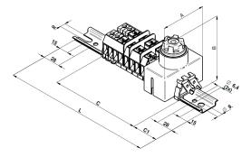
Fuse holders in pole terminal board systems do not include own fuse element (fuse DII) due to the varying requirements of customers for their own types of fuses. The E14 and E27 cut-out bases do not include a pressure insert (distance ring).
