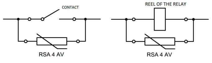
Example of RSA 4 AV connection in application of switching off voltage spikes. Example of RSA 4 AV connection in relay contactor protection application.
